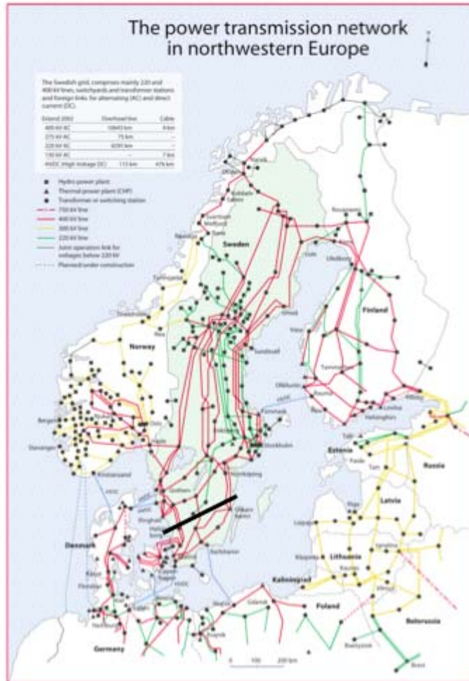
Fig. 1. The power transmission network in northwestern Europe. The line just north of Oskarshamn marks the modelled area.
