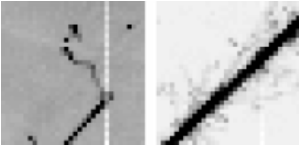
Figure 1. Examples of particle impacts on the ISOCAM instrument. On the left panel a low energy particle has probably stopped in the detector, while on the right panel a heavy ion passing through can be seen.
